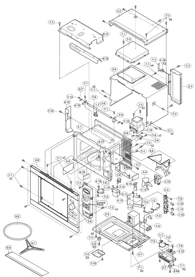
NOTE: In the event of removing the turntable motor cover this part should be refitted using screw connection: LX-CZA001WRE0 (7-15)
