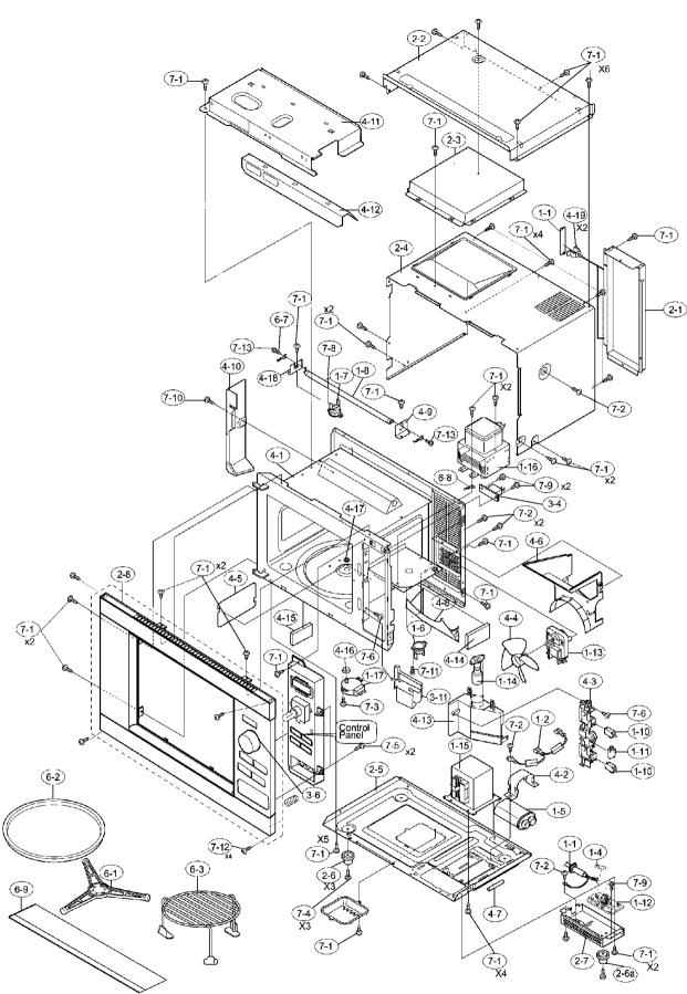
NOTE: In the event of removing the turntable motor cover this part should be refitted using screw connection: 50280576005 (7-1)
