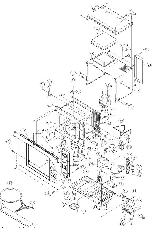
NOTE: In the event of removing the turntable motor cover this part should be refitted using screw connection: 50280577003 (7-15)
