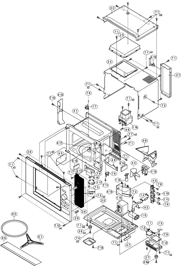
NOTE: In the event of removing the turntable motor cover this part should be refitted using screw connection: 50280576005 (7-15)
