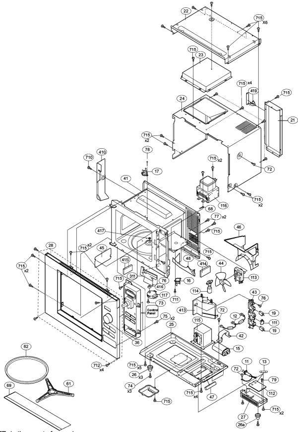
NOTE: In the event of removing the turntable motor cover this part should be refitted using screw connection: 5028 05 76-00/5 (715)
