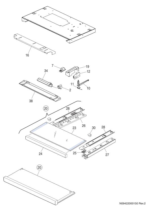
Notice: This exploded view is revised (Aug.31 2001) as well as the spareparts number. FRONT PANEL pos. nr. 24 can now acquire as a service kit (front panel w/ decor)
