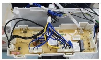
(1) When reasembling,once connect the connetors make sure the wiring inside the box. The wiring willnot cut by the sharpne part
