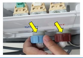
(2) Remove COLD/HOT WATER INLET HOSE
