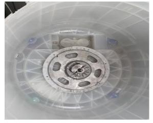
(8) Unscrew 2 screw which secure the plate assy
