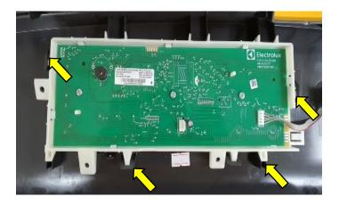
(4) Release the hooks which secure the display board (UI) to the control panel
