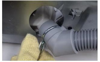
(2) Unscrew the screw which holding cover pump and take out the cover pump
