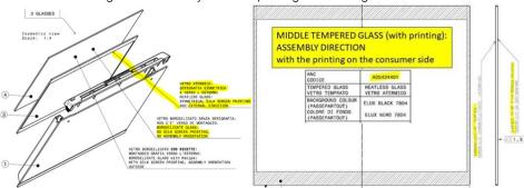
> To check the correct assembly of the cover (fully snapped-in) and the correct positioning of the glasses in the slots
