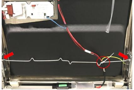
NOTE: Remember about the plastic badge that holds wire harness on the hinge rod – carefully pull out hinge rod from the badge – you can leave it on the wire harness as you will need to slide it back on the hinge rod.
