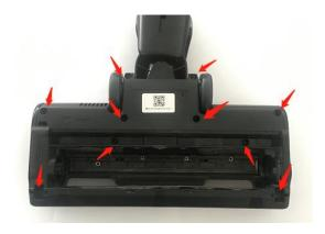
4.6 Remove left/right cover, take out top lid and BRC pedal
