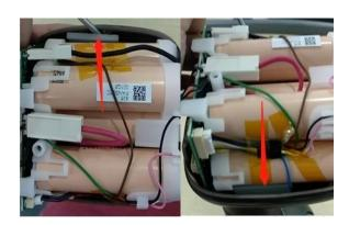
3.3.2 Unlock the terminals from PCBA,number 1 firstly(positive), number 2 secondly(negative), then for other terminals
