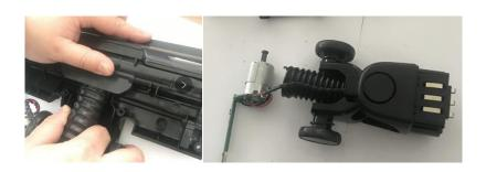
4.9 Use smaller flat screw driver to pry up the cover, unlock the screw to take out rear wheels
