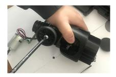
4.10 Use screwdriver to pry up the cover, unlock the screw, push up to remove the connector
