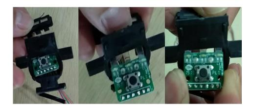
${\it 3.4.4 \ Disassemble \ motor \ assembly, take \ out \ suspension, \ \ unlock \ the \ 3pcs \ hooks (red \ arrow)}$
