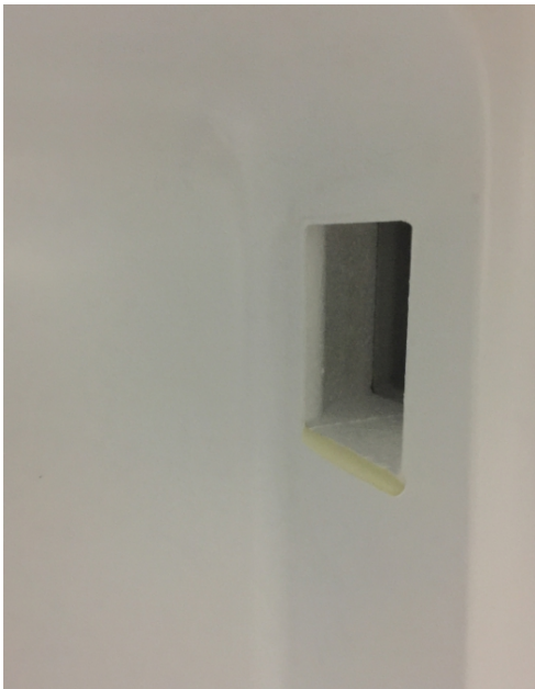
Air supply outlet freezer→cooler
