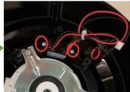
Remove the PCB, and unscrew two screws.
