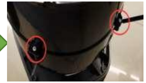
Remove the five screws from air duct.
