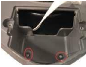
Unscrew two screws and take out the plastic part.
