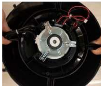
Remove the fan wheel part from the unit.
