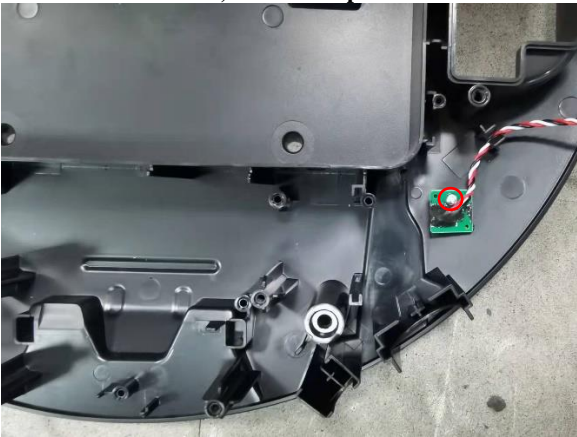
30.Remove the light guide
