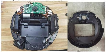
14.Unplug all the edges of the PCB board, take out the 3 screws shown in the picture, and remove the PCBA
