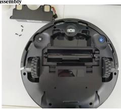
10. Unscrew 2 screws, take out the universal wheel shrapnel, universal wheel shaft sleeve
