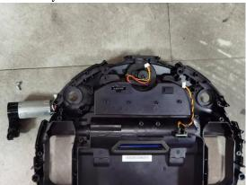
23. Take out the 2 screws shown in the picture, take out the infrared emitting bracket
