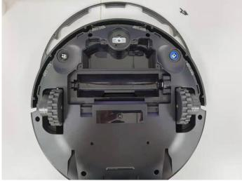
12. Remove the front bumper connector and remove the bumper assembly
