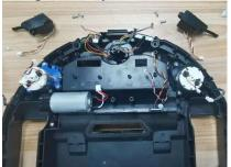
18.Unscrew the 6 screws and remove the side brush drive system left and side brush drive system right assembly
