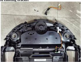
24.Take out one screw shown in the picture, take out the dust box induction PCBA
