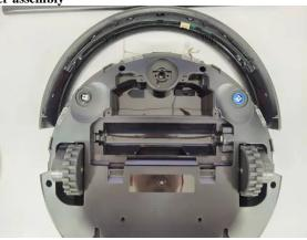
13. Remove the six screws in the position shown and separate the rear cover and base assembly
