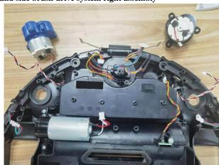
19. Tear off the rubber, and then remove the front impact shrapnel
