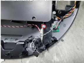
28.Remove one screw, remove water tank induction PCB
