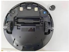
9. Remove the 4 screws, unplug the cable, and remove the battery assembly
