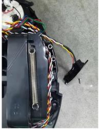
16.Unscrew the six screws and remove the left and right wheel assembly
