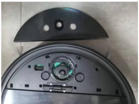
3. Remove the four screws from the pressure plate, take out the cover and lid
