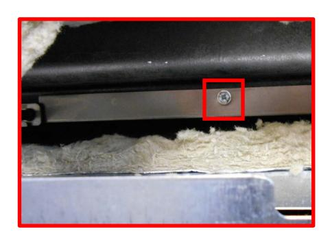
A tab at the centre of the element will require bending up
