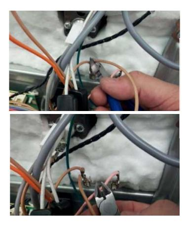
3. Cut the other end of the loose brown wire as close as possible to the fan element terminal and discard.
