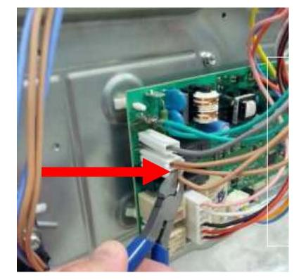
2. Cut the <u>single</u> Brown wire at the powerboard as close as possible to the terminal.
