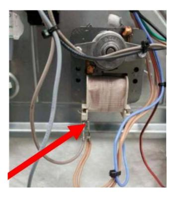
5. Connect the other Brown wire Double Piggy back terminal to the Brown of the fan motor.
