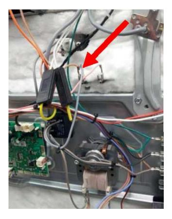
6. Connect the single Grey wire to the second terminal on the Fan element (Where the original brown wire was cut from in Step 3).
