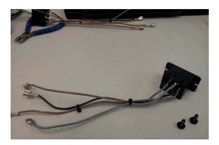
Kit consists of a relay, 4 wires, 2 screws and a klixon.
