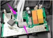
20. Insert motor and CW wire into main PCBA, fix the wire with slot, insert cooltube as picture shown
