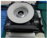
11. Put the sealing and bellow into motor housing rear
