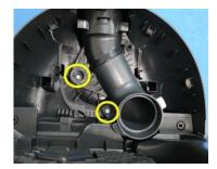
27. Assemble cover front and under into base and make sure slot in place, fix with 2pcs screws
