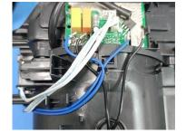
21. Insert the sealing into motor housing
