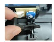
18. Insert the wire into on/off switch PCBA and fix it in motor housing
