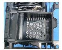
22. Insert sealing and cootube into air channel, assemble air channel into base as picture shown
