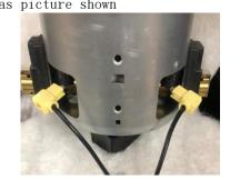
10. Diffusor wrap the motor and put it into motor housing, then install suspension ring
