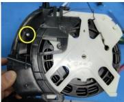
15. Assemble CW/motor housing rear with motor housing front and pull out the wire from bracket, keep the clip in position, fix it with 4pcs screw
