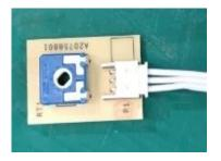
17. Insert the knob pin into the hole of PCBA
