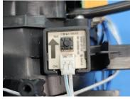
19.Install the main pcba into base and fix the clip angle, insert the wire of potentiometer and on/off switch into mani pcba
