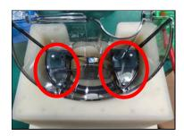
3. Put the sealing into lid, fix the spring as below and assemble the catch into lid, put the lid into dust bin
