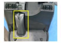
29. Install the cyclone assy into base and fix with 6pcs screw
