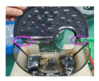
4. Put the sealing into cyclone, put the nose cone into cyclone, pay attention to the slot postion
