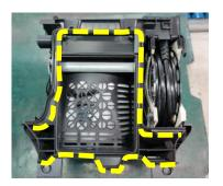
26. Install the motor housing assy into base, check all sides are located in postion, fix with 2 pcs screws
