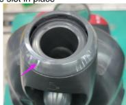
31. Insert button ino lid, fix spring into cover and fix cover into lid with 2pcs screws
