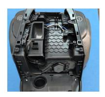
7. Remove the cover under with screw, then using the tools to disassemble the cover
