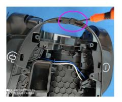
13. Use the flat driver to remove the clip and right cover
