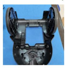
11. Use the flat head driver to remove the clip of left cover
