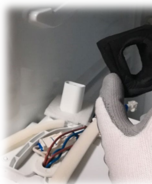
6. Remove the silicon tube and sealing sponge
