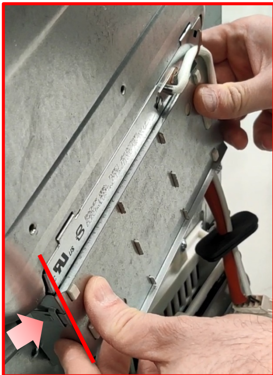
Too much pressure on assembly create deformation
