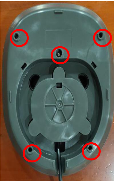
11. Remove 5 screws of the Base Cover
