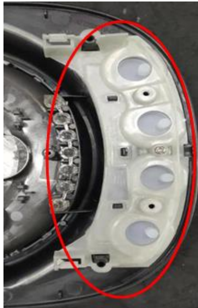
16. Disassemble the Press Key (WHITE)
