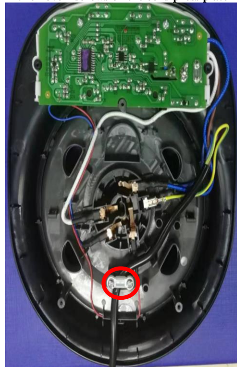
12. Remove 2 screws on the cord press plate
