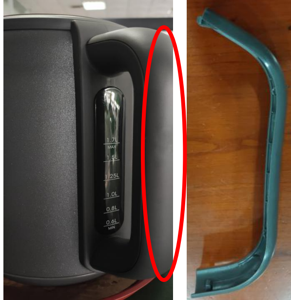
2. Disassembling the Handle Upper cover
