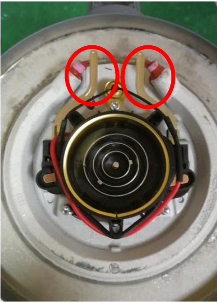
5. Pull down the Thermostatic connector
