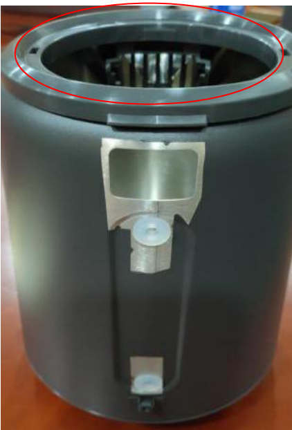
7. Disassembling the Spout cover
