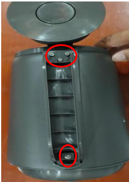
3. Remove the 4 screws of Lower Handle cover
