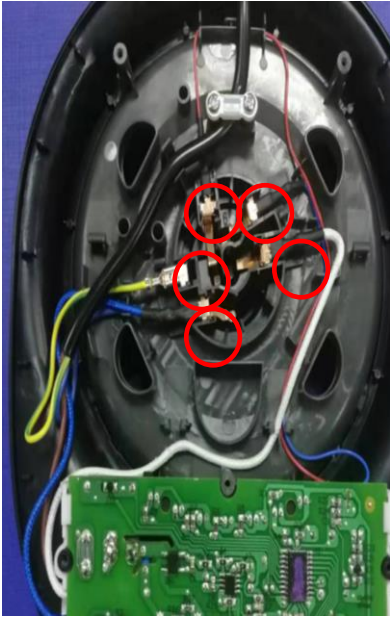
13. Pull down the Lead wire Terminal
