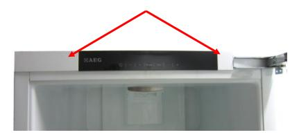
3. Remove two screws and pull out the electronic.
