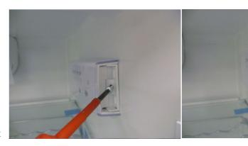
Remove the screw and take out the control unit
