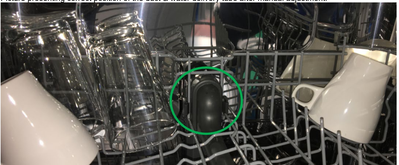
Picture presenting correct position of the duct & water delivery tube after manual adjustment:
