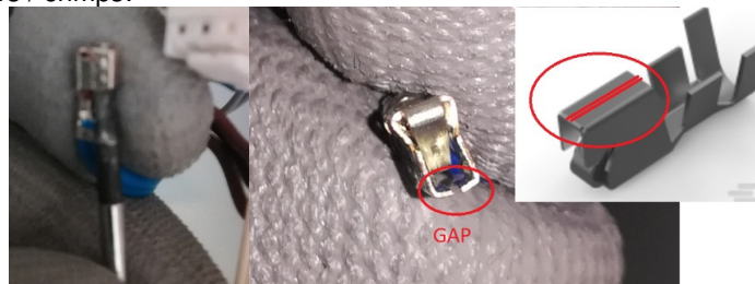
Gap between metal connector on the top surface
