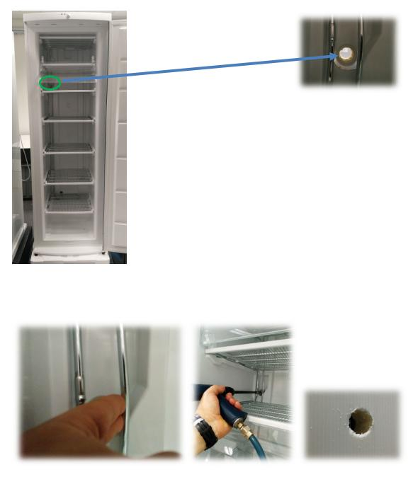
2/3 Insert the valve and re-align the tubes.
