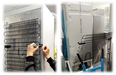
2/2 Carefully bend the tubes and drill a Ø27mm hole in the inner liner.
