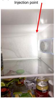
Empty the refrigerant system. Reload with gas and close it.
