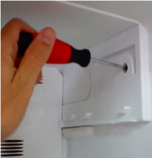
Unscrew the screw fixing the freezer partition. (KA 40*14 WN 1411(INOX) EJOT)
