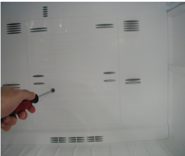
Remove the drain pan plug. Unscrew the screw fixing the freezer multiflow cover. (KA 40*14 WN 1411(INOX) EJOT)
