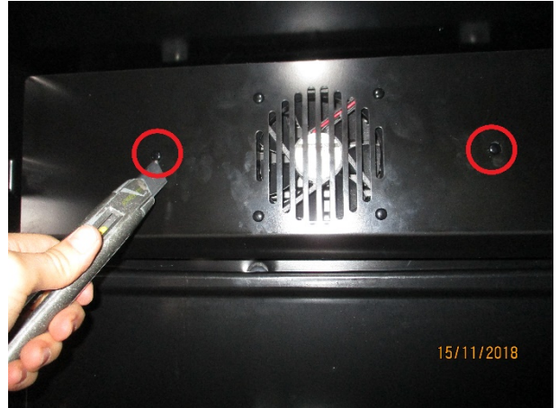
7) Open the door, remove the grids and unscrew the 2 rivets that fix the evaporator protection
