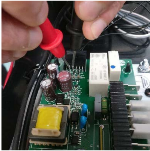
Fig. 4 (Voltage tested in DC between second and third pin from the left: around
