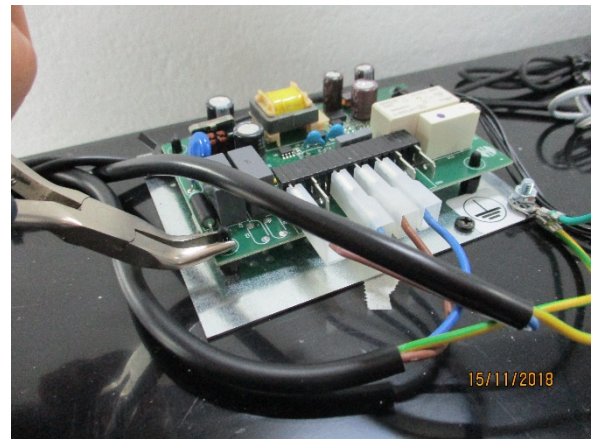
4) Use a clamp to uscrew the PCB from the 4 interlockings
