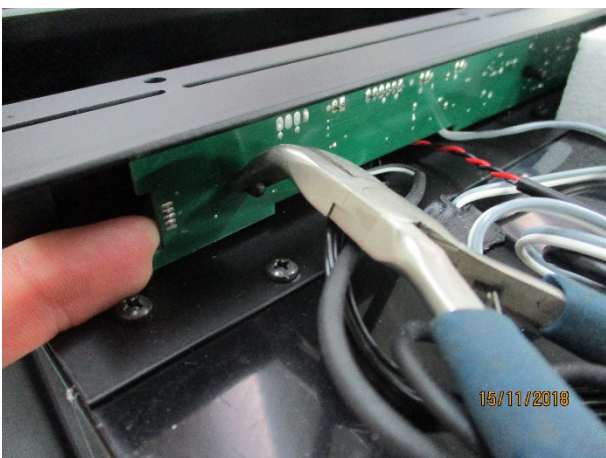
5) Use a clamp to unscrew the display from the 3 interlockings
