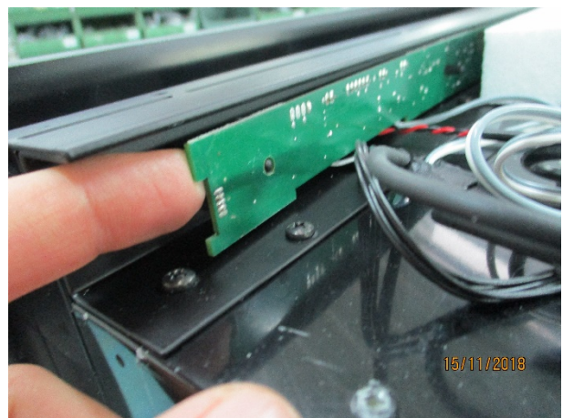
5) Use a clamp to remove the 3 interlockings that fix the display
