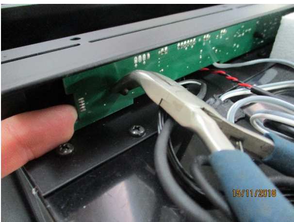
5) Use a clamp to remove the 3 interlockings that fix the display
