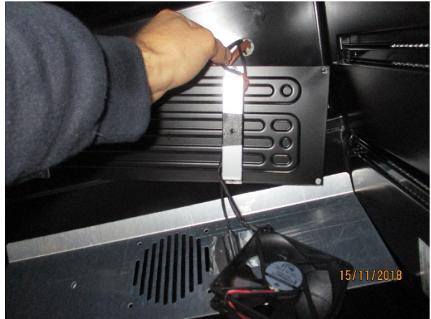
9) Move the evaporator and pull the fan connector
