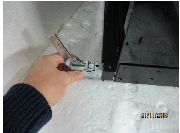
4) Pull out the hinge and replace it with a new one
