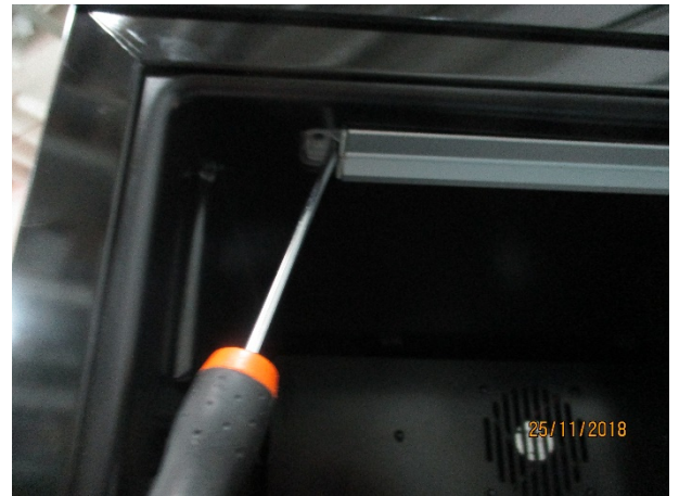
9) Use a screwdriver as a leverage to remove the led bar
