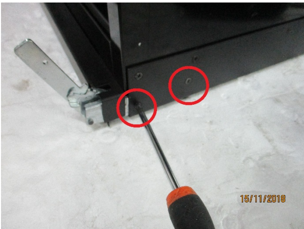
3) Unscrew the 2 screws that fix the door hinge
