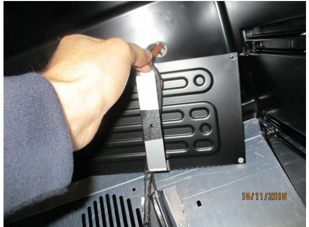
9) Move the evaporator and pull the NTC wire
