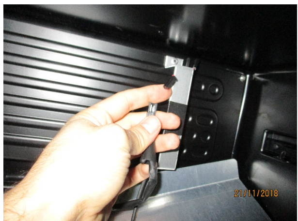
10) Disconnect the fan connector from the fan, and replace it with a new one. Then reverse the procedure to install the connector
