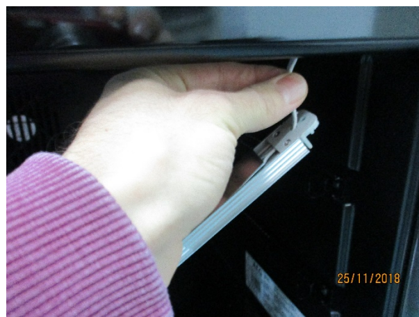
10) Pull the display connector, and reverse the procedure replacing the led bar with a new one
