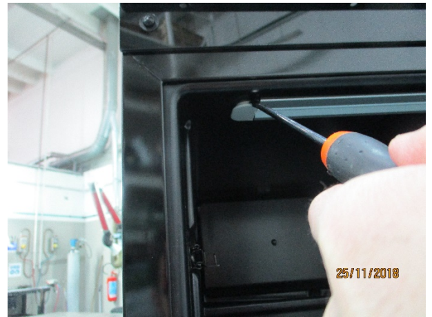
7) Use a screwdriver as a leverage to remove the cap (from both sides)
