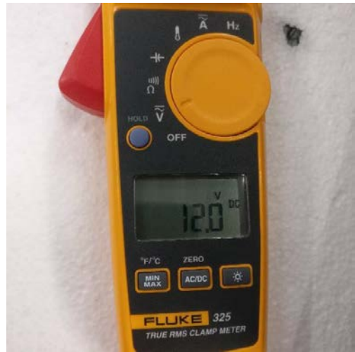
Fig. 4 (Voltage tested in DC between second and third pin from the left: around
