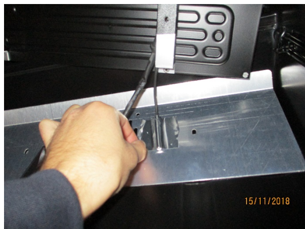
10) Detach the sticker that fix the NTC, and then reverse the procedure replacing the NTC with a new one
