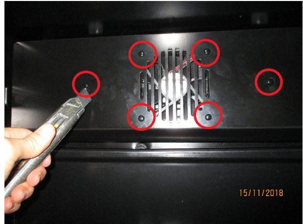
7) Open the door, remove the grid and unscrew the 6 rivets that fix the evaporator protection and the fan
