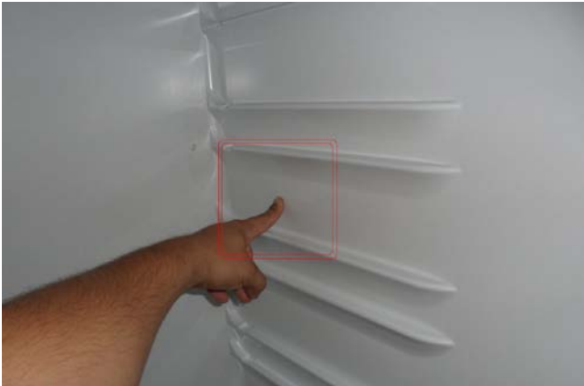
Probe position on the refrigerator evaporator (not replaceable)
