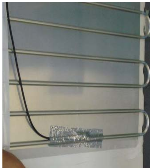
Probe position on the refrigerator evaporator (not replaceable)
