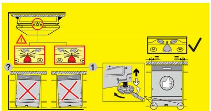
b) The diamond should be at least levelled or higher than door lock catchers. If it remains below the hooks, the inner door or the upper cross bar has been deformed.
