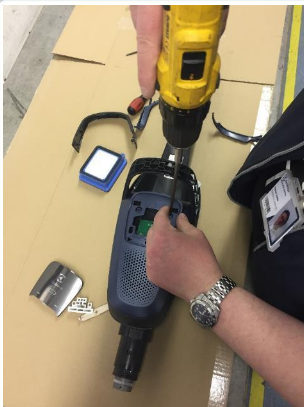
Remove the 3 screws from the lid.
