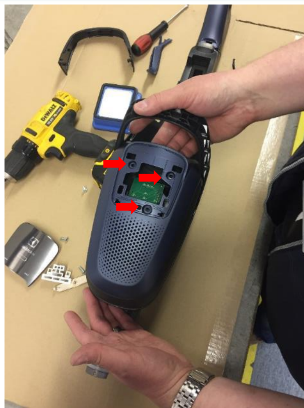
Remove the 3 screws from the lid.
