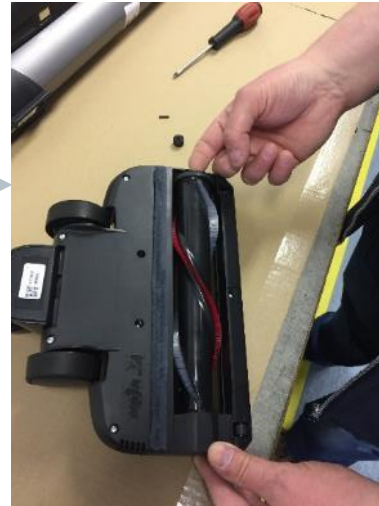
Remove the brushroll from the nozzle.
