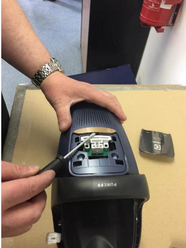
Snap out the lid decor with a screwdriver.
