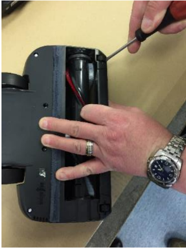
Remove the front wheel with a screwdriver.
