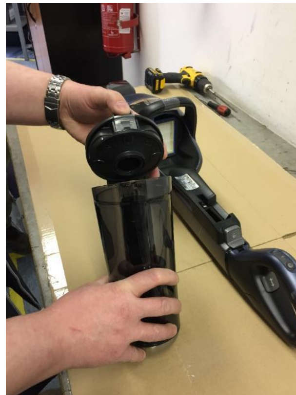
Open the dust container filter.
