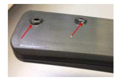
Spray arm nozzles damaged because of collision with Lower Rack
