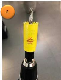
2. Drill a hole with a 27mm drill to the left side of the inner liner.
