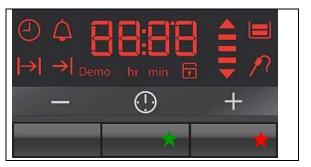
I. Press long the +" $\star$ " key. Demo indication and the  $1^{st}$ . Digit is blinking.
