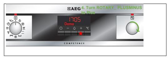
3. The +"★" key is still pressed. Turn temperature selector right until buzzer sounds 3x. On the display appears Demo
