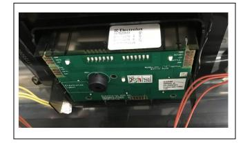
Remove the rast connectors from the User Interface
