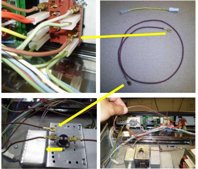
5 - Identify and disconnect the yellow wire that connect terminal (2) of the switch. Connect it to the protected male terminal of the additional yellow wire.
