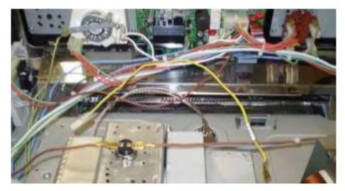
4 - Connect one side of the additional brown wire in the terminal (b) of the switch. The other side must be connected to the thermal protection of the magnetron.
