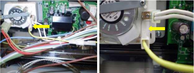
7 - Connect the brown wire that comes from the digital programmer (previously connected to thermal protection of magnetron) in the terminal (2) of the switch.
