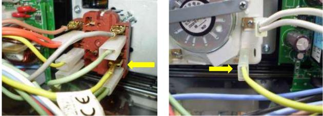
3 - the yellow bridge from the wiring. Cut one of the terminals and pull the yellow from the plastic cable tie.
