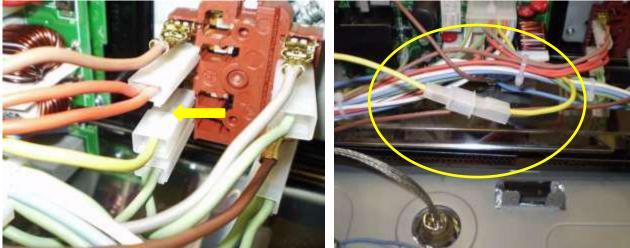
6 - Connect the other terminal of the yellow wire in terminal (2) of the timer.
