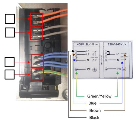
**Terminal block Internal Connection**
