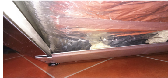
Insulation on the underside of oven is settling on the trucking plate
