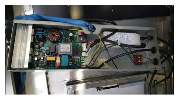
5. Disconnect all cables and remove the board from the box (pay attention to the pins in the circles)
