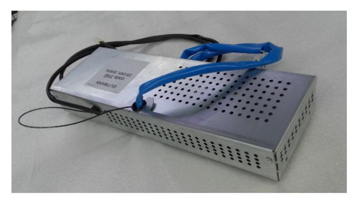
12. Fix the trasfromer, the terminal block, the ground connection and the main board (see picture).
