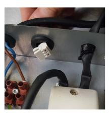
8. Remove the ground connection and the terminal block
