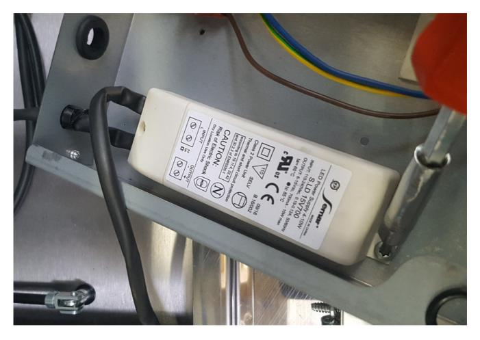
10. Disconnect the wires in the transformer in order to remove the trasformer from the box
