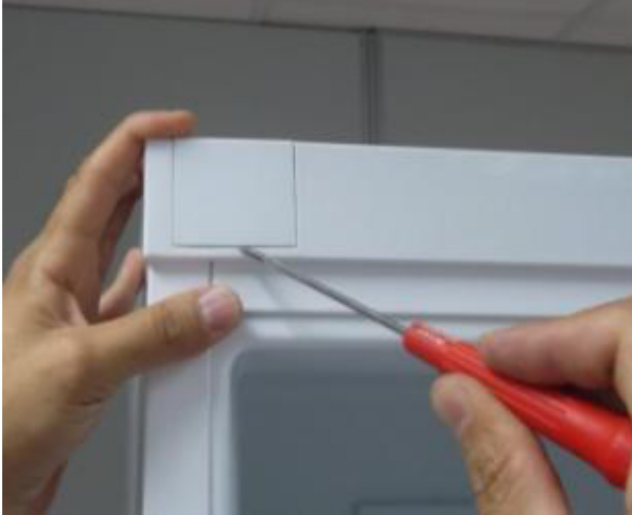
1. Remove the panel cap by the help of the slotted Screwdriver
