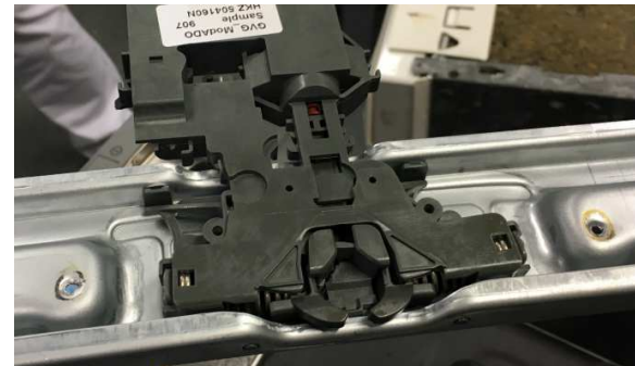
Detail of the snapped fixation with 2 screws on the upper front cross bar
