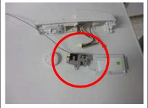
7.Assemble the control unit with the new thermostat and place it back
