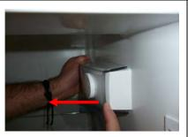
2.Remove the light bulb then unhook the control unit with the help of a screwdriver
