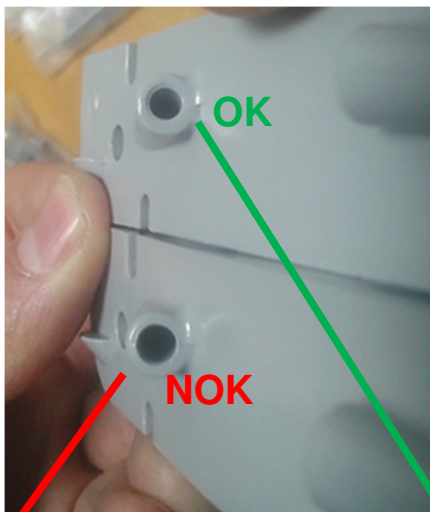
Photo 1. Water distributor nozzles.
