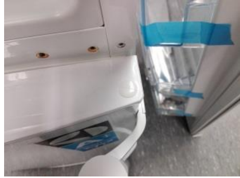
12. Dismount freezer door. Disassemble lower hinge.
