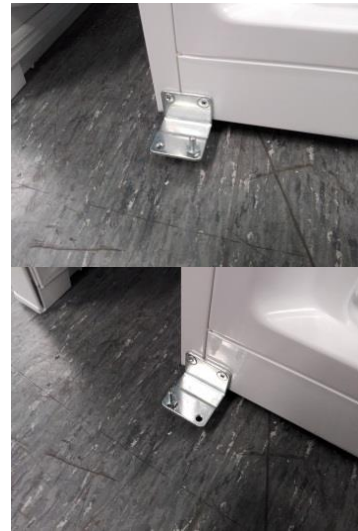
14. Place and fix lower hinge then place pivot on opposite side. Later reattach freezer door.
