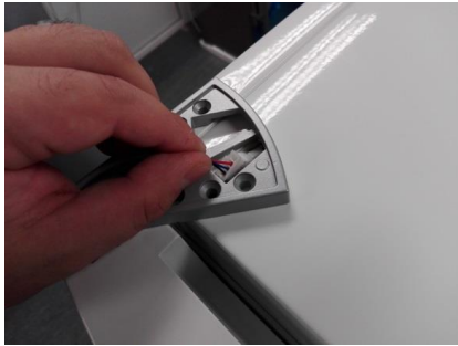
17. Place upper hinge on opposite side then adjust wire. Pull out carefully connector from box. Pair connectors and place joint back into box. Fix hinge with screws. Put back plastic cover onto hinge.
