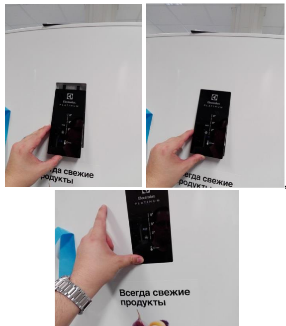
19. Assemble LCD back in door.
