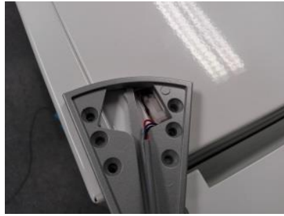
17. Place upper hinge on opposite side then adjust wire. Pull out carefully connector from box. Pair connectors and place joint back into box. Fix hinge with screws. Put back plastic cover onto hinge.
