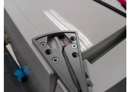
17. Place upper hinge on opposite side then adjust wire. Pull out carefully connector from box. Pair connectors and place joint back into box. Fix hinge with screws. Put back plastic cover onto hinge.
