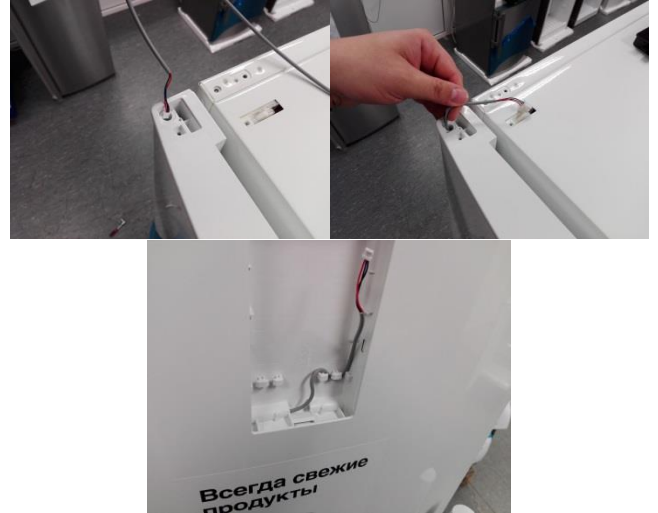
16. Place back fridge door then push wire back through the channel. Adjust wire in the LCD's bay.
