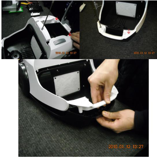
3. Take out the 4 screws, and remove the motor house!
