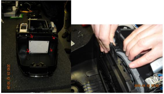
4. Remove the blower seal, after that, you can take out the motor. The Cord winder is assembled to the right side of the motor house.
