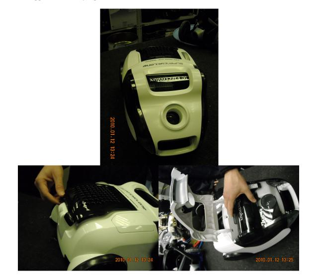
1. You have to remove the grill filter from the back side of the cleaner. After that the dust container cover is easily removable. Open the cover, and push the lock on the both side, and pull the cover in direction of the front side of the cleaner!
