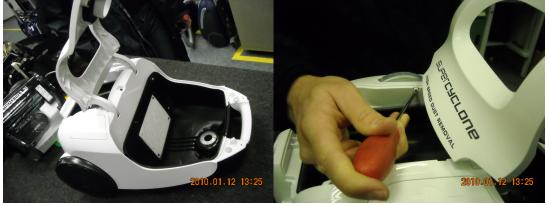
2. Remove the 3 screws on the back, and 2 screws on the front side of the cleaner. After that, you can easily lift up the rear cover. After that you can find the Pcb, below the left side of the rear cover.
