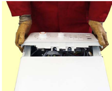
Remove the control panel (see service manual).
