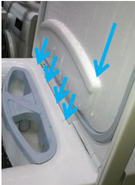
Photo1. Water dripping from opened lid into the gap between top part and lid.
