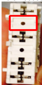
4. Identify the part of plastic housing that needs to be removed. It is located between two single pins.
