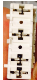
3. Simplified version of OVC3000 and corresponding connector (4 pin). Direct replacement not possible. Cable modifications necessary.
