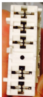
2. Fully equipped OVC3000 and corresponding connector (5 pin). Replacement can be used without any additional operations.
