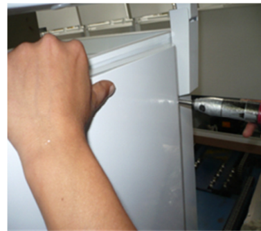
6. Screw back the low frost cover
