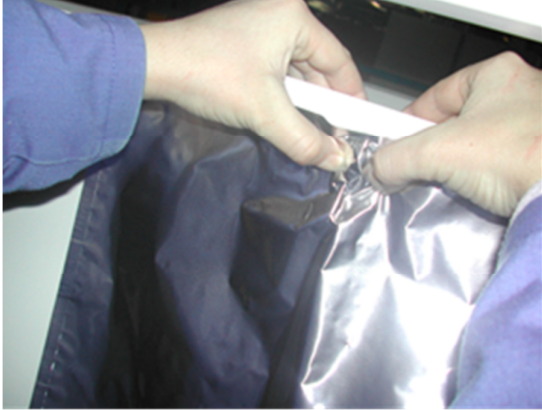
3. Check bag and plastic tube if they are damaged.
