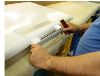
11. In case of AEG brand – attach the decor plate
