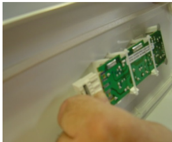
8. In case of handle with electronic PCB, attach old electronic to new handle and connect it
