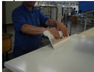
9. Assembly the electronic to the lid
