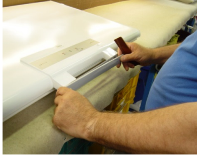
3. Remove the decor plate (only in AEG)
