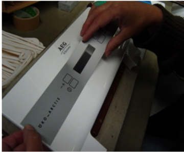
5. Remove handle from lid. In case of electronic version disconnect the electronic board
