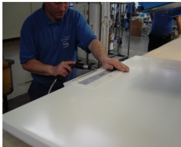
10. Fix the handle with 2 screws
