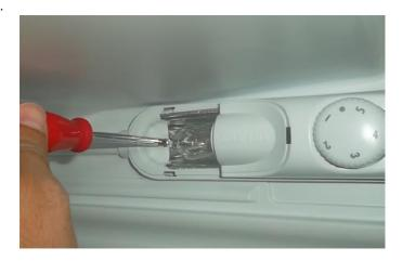
4. Assemble the new lamp cover by placing the detail to the housing.
